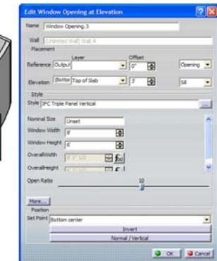
4. You should have 6 windows on the curved wall between 2 doors. Place a window on the west wall using the center point as “Reference”. Choose “IFC Triple Panel Vertical” within “Windows > IFC Standard Windows”. Under “Elevation” set the “Offset” to 3”. Set “Window Width” to 8” and “Window Height” to 6”. Click OK.
