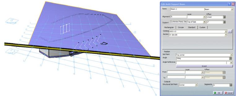
2. Press the “Standard” tab and click the “...” button. Press the “Current” drop down menu and choose “AISCv13 catalog”. Double click “W (Structure Design)” and then “W 18x106”. Click OK. The beam will be extending into infinity until we create the other beams to limit it.
