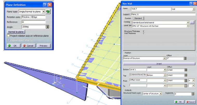
3. Select the “Level 1” grid level for “Bottom”, the southern perimeter beam for “Top” with “Layer” set to “Bottom” and the output line “Offset West” under the sketch “Partitions > Outputs” for “From”. Click OK. Choose the “Wall” tool and setup the “Support” plane for the western perimeter.
