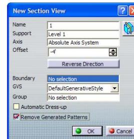
4. Click OK. You should now see your plan cut in the model view at the location it’s being generated. To see the steel beams above create another “Section View”. Name it “RCP”. Set “Support”, “Axis” and “Offset” the same as before. Change the “GVS” to “RCP”. Make sure to uncheck “Automatic Dress-up”. Click OK.
