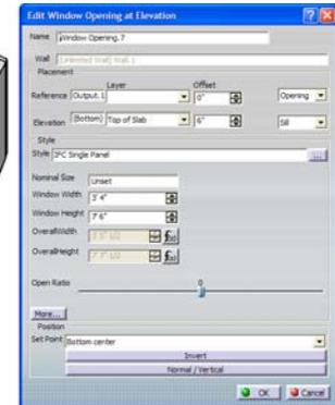
2. Under “Elevation” click the “Layer” tab and select “Top of Slab” (even if this option is already selected). Set the “Offset” to 6”. Set the “Window Width” to 3’4” and the “Window Height” to 7’6”. Confirm the “Set Point” under “Position” is set to “Bottom center”. Click OK.
