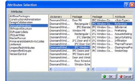
2. First we need to set the window tag data. Search (Ctrl + F) for “IFC Window Common Properties”. Press “Excel Data Sheet” and click “Report...” under “Attributes”. Select “DoorsandWindows > IFC Window Common Properties > Reference”. Click Apply. Enter “I40A” for 1-6 and “I96A” for entry 7. Click “->Synchronize<-” and OK.
