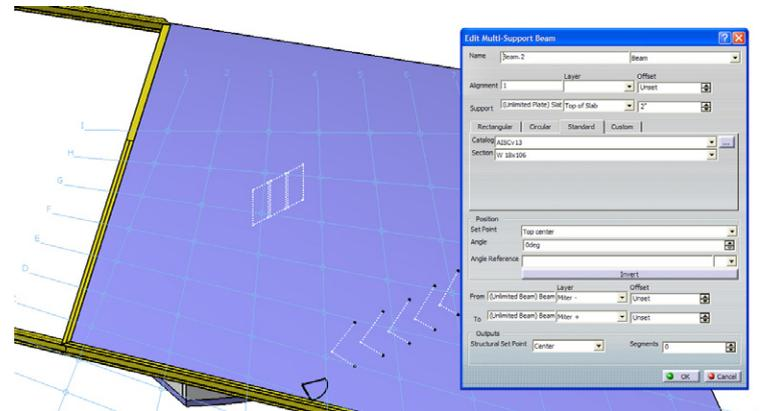
4. Create the third beam from the “I” east-west running grid axis and choose the previous beam for “From” with “Layer” set to “Miter +”. Click OK. Double click the second beam to edit and set the “To” field to the third beam. The “Layer” drop down menu will default to “Miter +”.
