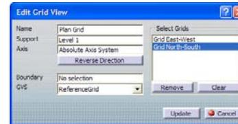
3. Click “GridView” again. This time name it “Elevation Grid”. Set “Support” to the vertical plane created for the section view. “Axis” is the same as before. Set “GVS” to “ElevationGrid” and select the “Building Levels” elevation planes under “Select Grids”. Click OK. Return to drawing and “Superpose” “Elevation Grid” to “2” view.
